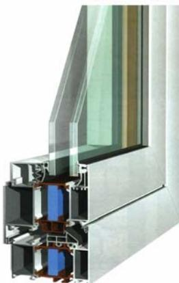
For this window system the thermal resistant barrier is achieved with a polyamide bridge of 32-36 mm. Furthermore, the interior air space is filled with expanded polyurethane insulation to greater enhance the thermal resistance of the system. The system also uses specially designed gaskets for improved weather resistance.
