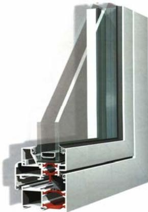
This window system is provided with a thermal resistant barrier that is achieved with a polyamide bridge of 18 mm.
